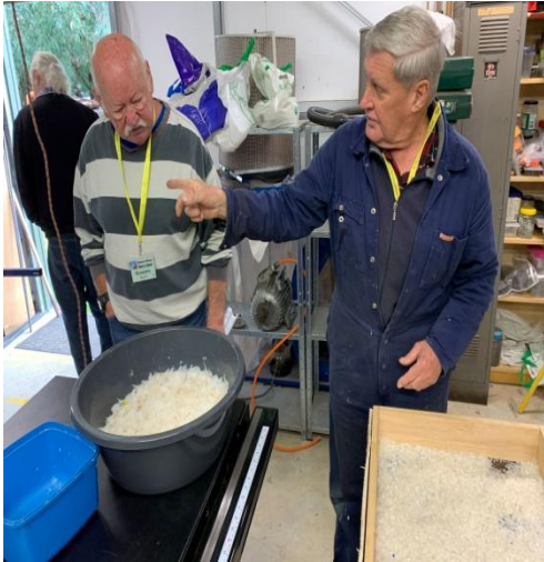
1- Finely ground milk bottles are dried to remove any water.
